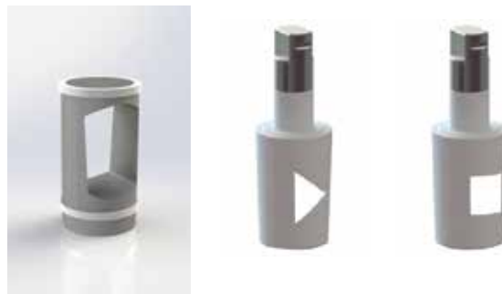
Figure 2: Control Plugs, fully PTFE lined with equal percentage and linear characteristics.
