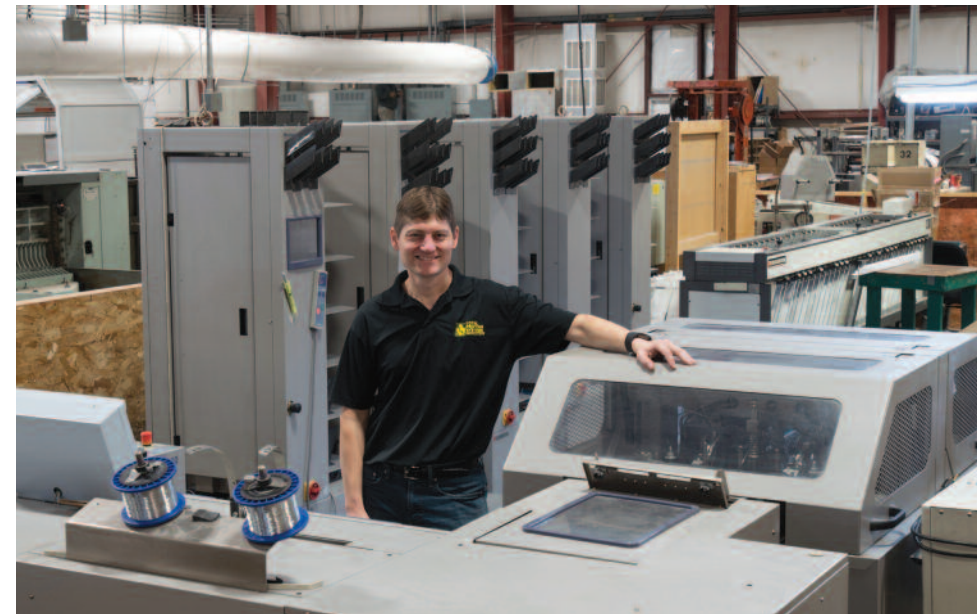
President Rick Lindemann of Total Printing Systems stands beside their Standard Horizon StitchLiner 5500 Saddlestitcher, which is used to produce a wide range of booklets for customers whose needs include educational workbooks, training manuals, and religious pamphlets.
