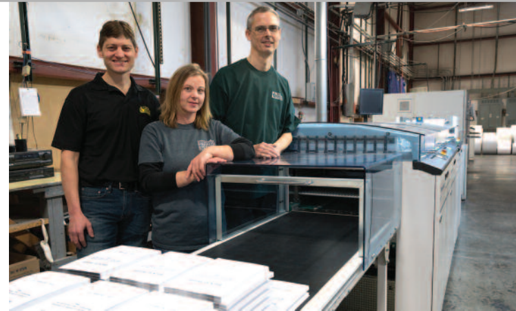
The team at TPS reviews the offset stacks being delivered for perfect binding from one of two Standard Hunkeler Roll-to-Stack Systems.
