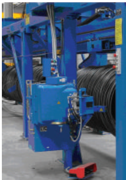
▲ The Type 3a slewable butt welding machine, mounted on a column
