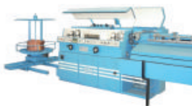
▲ The model HS6H with hydraulic and flying shear cut for wires from 1.5 to 6mm
