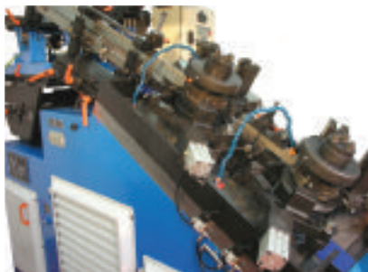
▲ The VA20/20-ESS for thread rolling of hi-tensile fasteners
