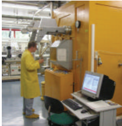
▲ Operator using the indentation tester in a hot cell
