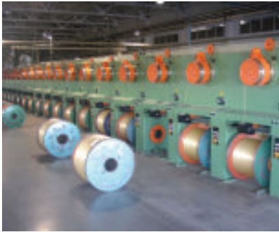
▲ Spool take-up frame with double accumulation capstan for non-stop operation
