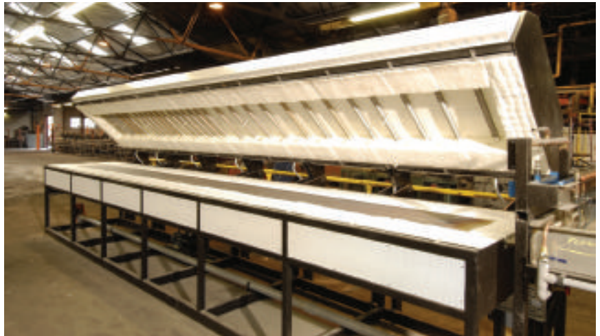
▲ Meltech's electrically heated furnace
