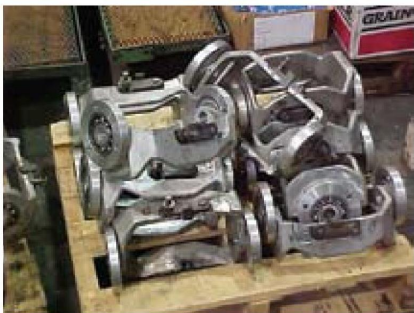
▲ Figure 2: Machine is completely disassembled and cleaned and the old bearings removed
