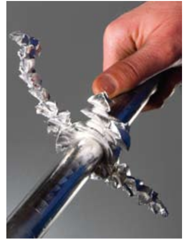
▲ Flash photo: Close up of an aluminium weld showing the resulting flash where the excess material, and any impurities, has been squeezed out from the interfaces
