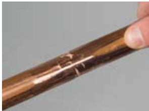
▲ Close-up weld: Close up of a cold weld on copper rod after deflashing and rubbing down ready for the drawing machine
