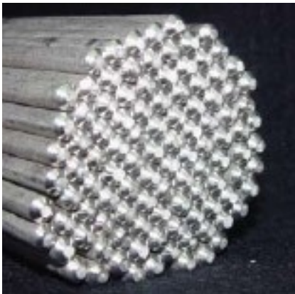
▲ Chamfered rods using Videx technology
