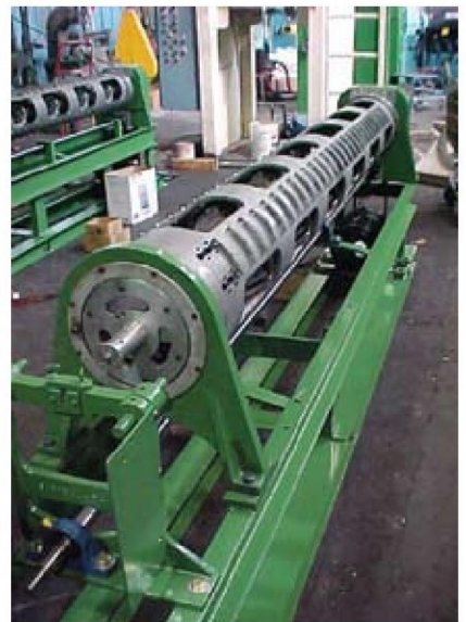
▲ Figure 4: Drive shaft aligned, cradles and wire guides are reinstalled and the cradle assembly is completed
