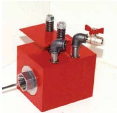
▲ Wire rod lubrication by PDH system
