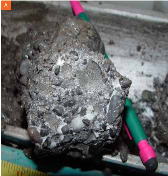
In sands and other coarse-grained sediment, gas hydrate (white) can form between the sediment grains (dark grains) as shown in this example from the Canadian Arctic.
