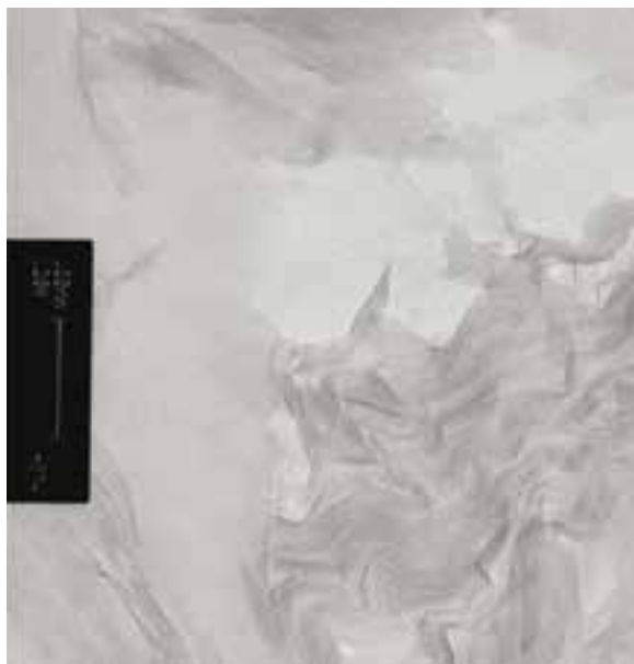
Figure 2: TEM micrograph of “Cloisite 25A” NCs at 5% concentration (bar size – 20 nm).
