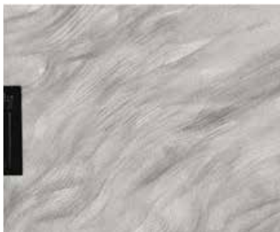
Figure 1: TEM micrograph of Nano1 NCs at 3% concentration (bar size – 20 nm).
