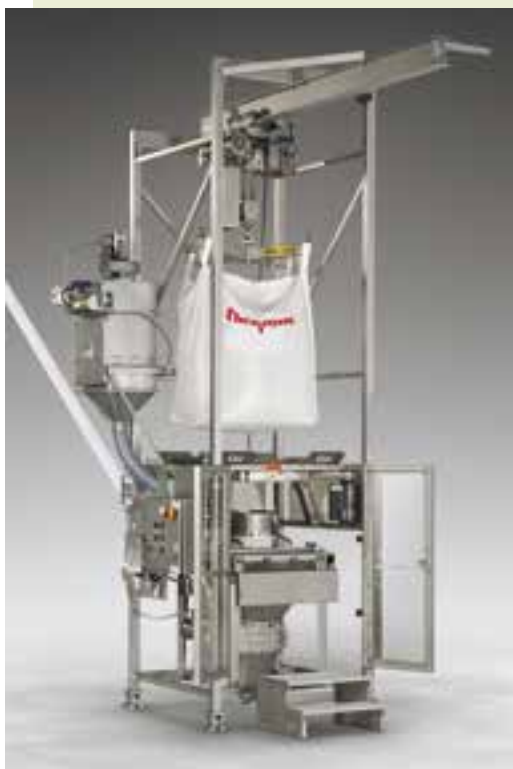
BULK-OUT™ Sanitary Bulk Bag Weigh Batch Unloading System with integral flexible screw conveyor and BAG-VAC™ dust collector shown with safety interlocked doors in open position and manual dumping station bag tray in lowered position.
