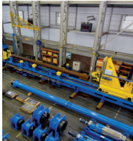
The Fontijne Grotnes pipe expander
