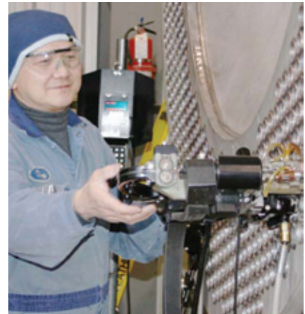
Orbital tube-tubesheet welding (above and below)
