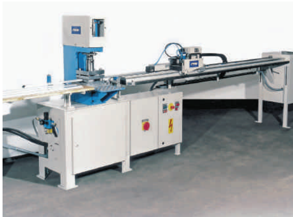
Figure 1: Petig's range of tube punching machines utilise the through-punching method
