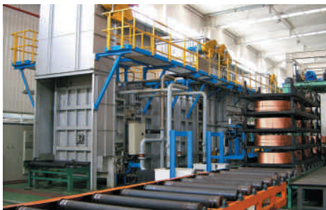
Figure 10: 5t/h stacker type furnace for the annealing of level wound copper tube coils
