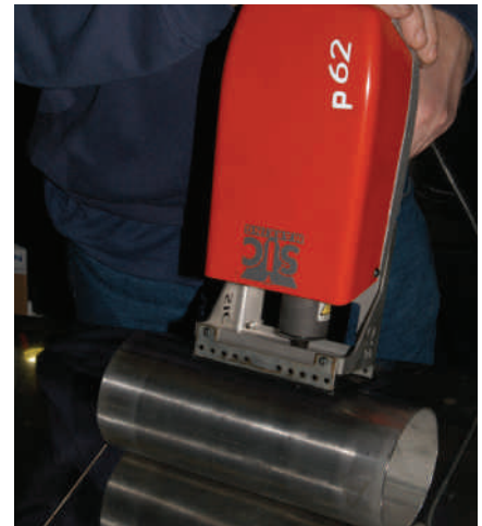
UMS manufactures a range of SIC portable dot markers for tube and pipe
