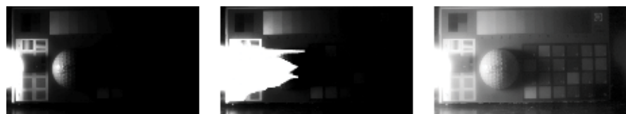
איור 2. A scene with both bright and very dark components, imaged by a standard IT-CCD (left), a standard EMCCD (center), and an Interline Transfer EMCCD device (right)
