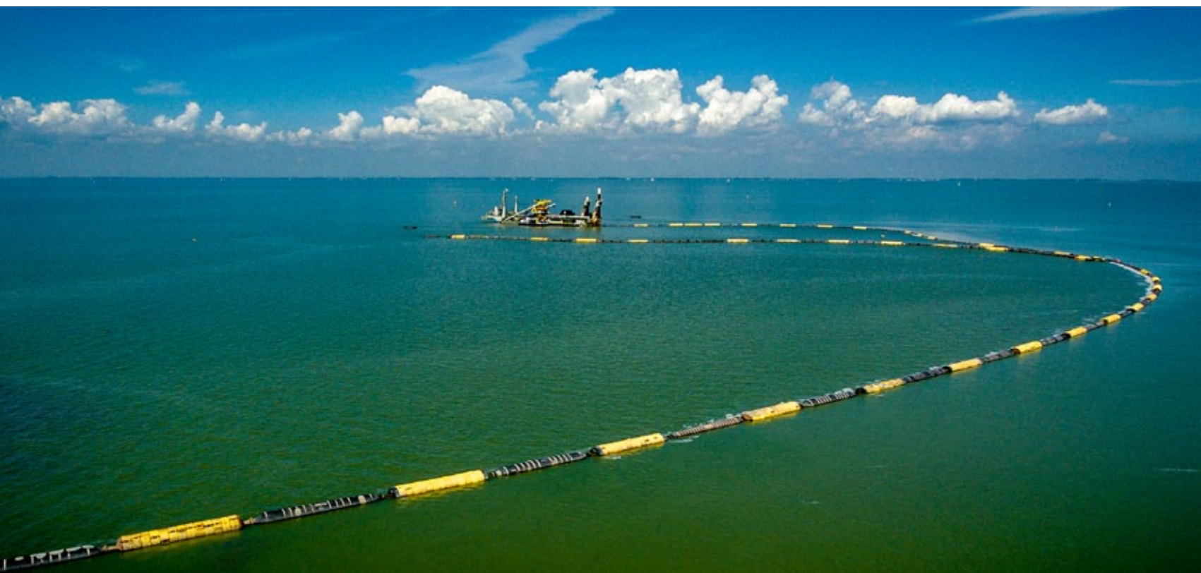
Cutter suction dredger Edax operating on biofuel on the Marker Wadden project.
