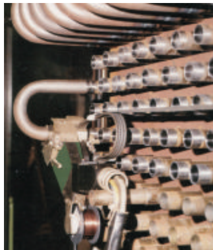
M34 for TIG welding tube-to-tube with filler wire
