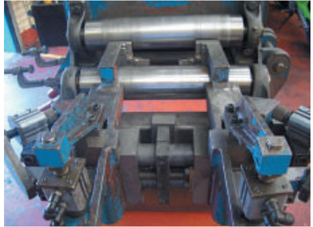
A close-up of the new strip edge preparation unit
