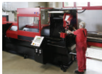
Ⓜ Circular saw for tubes and solid bars up to 170mm diameter
