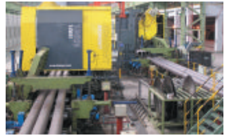
Linsinger's KSA 1600 carbide circular saw
