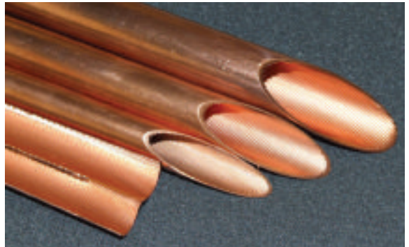
A section of inner grooved copper tube
