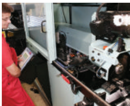
Ⓜ Multicut saw for short length tubes of 30 up to 100mm fixed length
