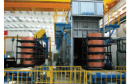
The entry end of an indirect gas fired roller hearth furnace
