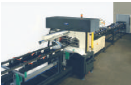
② Petig's combined section and tube stamping machine for open C-sections
