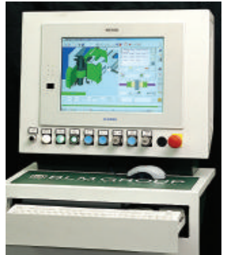
BLM Group's VGP3D software automatically selects the tube bending program parameters to optimise cycle times
