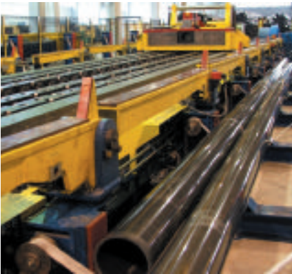
Ⓣ Cartacci builds draw benches with drawing forces of up to 300t
