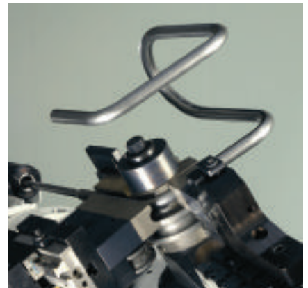
Creating a tube bending program is fast and easy with the 3D graphical programming facility provided by VGP3D software
