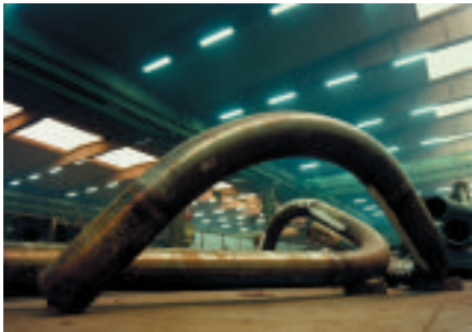
Ⓣ Fabricom GTI can create bends in multiple planes from a single length of straight pipe
