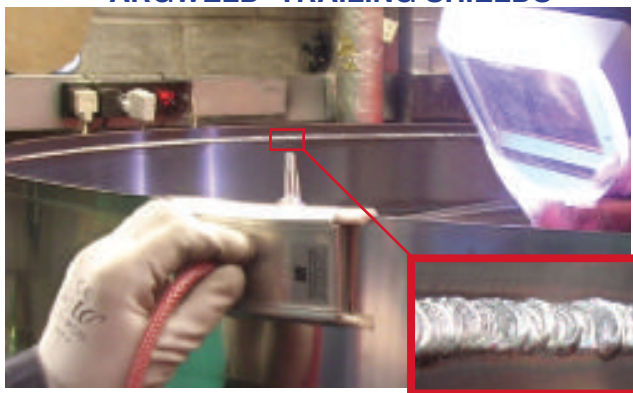
OD and ID Argweld® Trailing shields working together allow for a simultaneous top and back purge on a stainless steel vessel.
