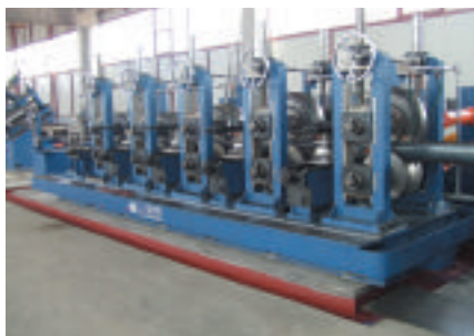
The 8" tube line's forming stands
