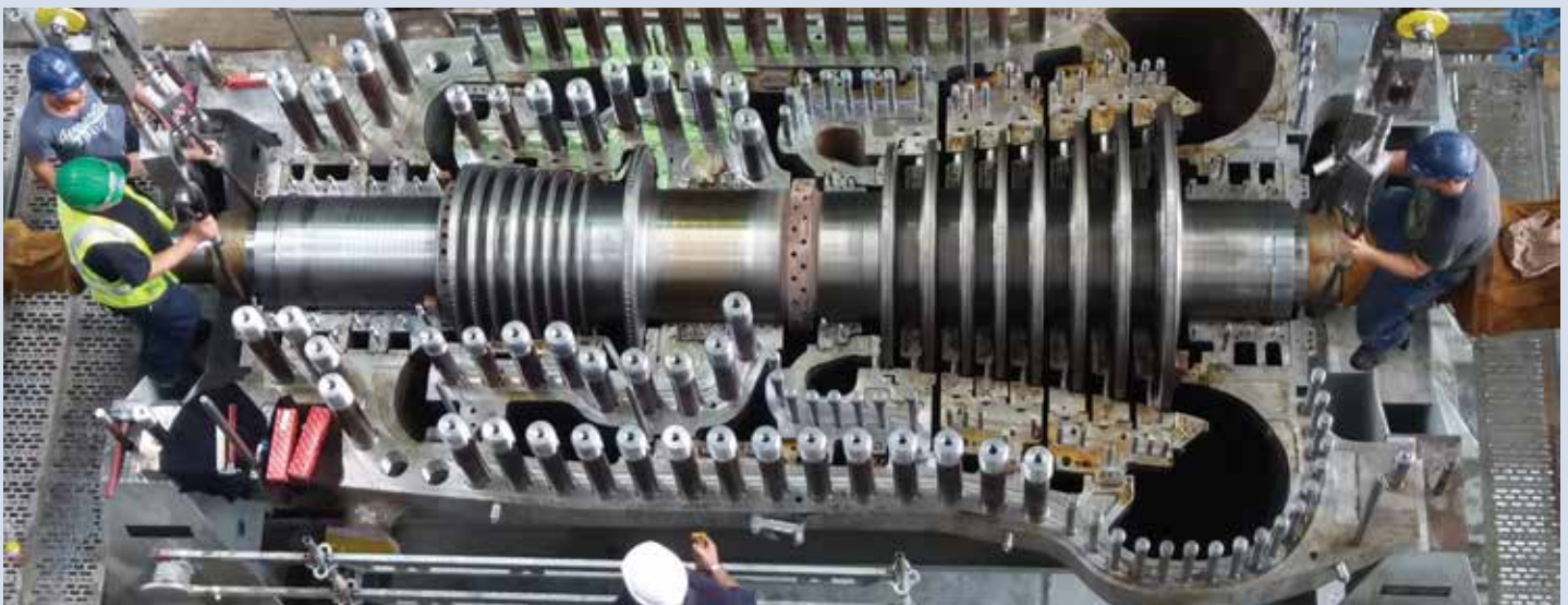
Actom Turbo Machines fitting the 15 ton, 150 MW Skoda Doosan turbine rotor.
