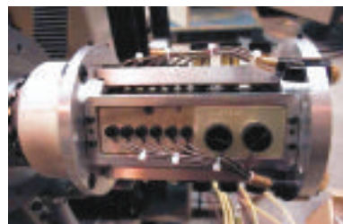
○ Example from rebuilding to up-grading: CARB bearings on double twist machines and quick change brushes holder on slip rings
