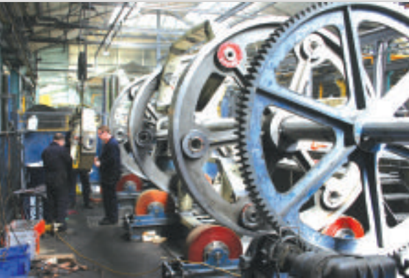
○ Re-assembly of refurbished bobbin cradles
