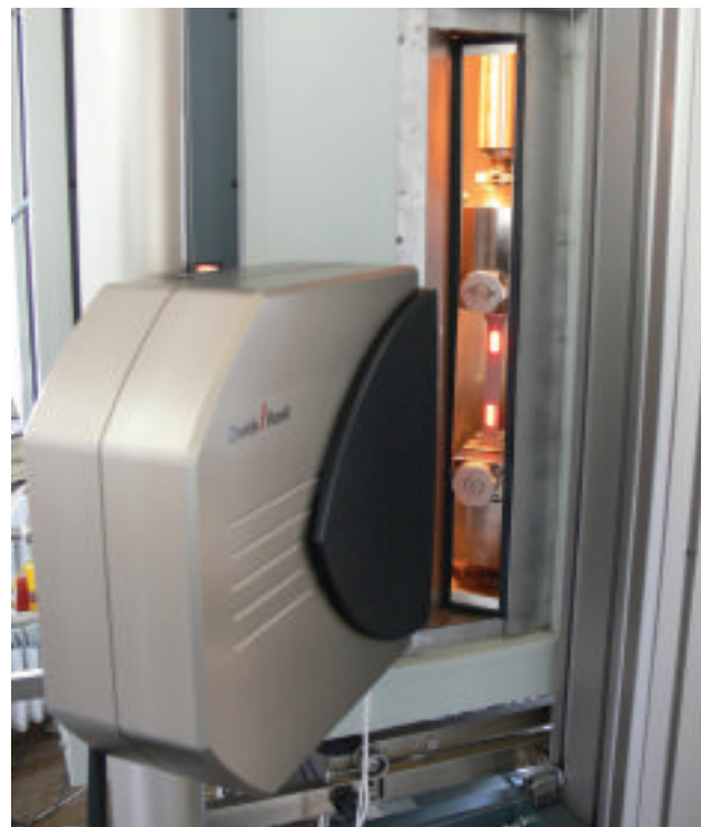
○ Extreme temperatures tested the new strain measurement system
