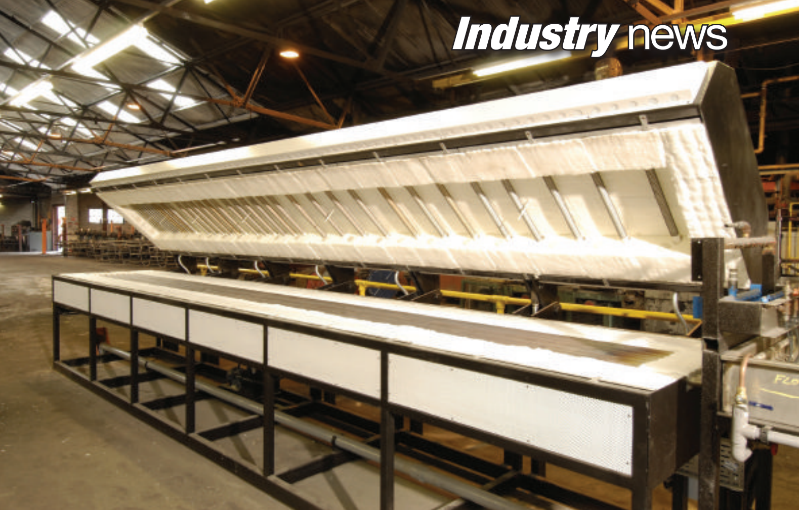
○ Meltech's electrically heated furnace
