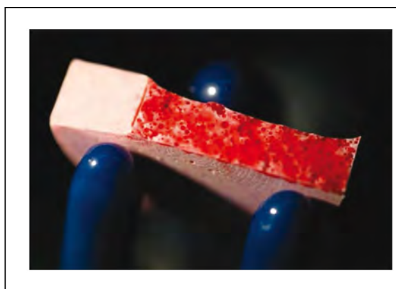
Figure 11: Close-up image of one-half of a self-healing epoxy specimen after it has been fractured into two pieces (Magnus Andersson, University of Illinois).
