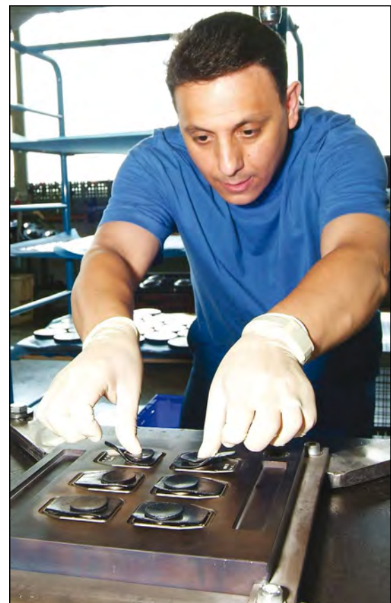
Preparation of EPDM diaphragms for vulcanisation
