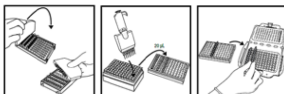
Figure 2013.09C. Transfer of lysate to reagent tube.
