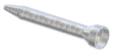
All mixer nozzles are industrial grade safe to 100psi and silicone free plastics. Manufactured from high density polypropylene with white mix elements. Total length of 379mm. The end is stepped with a 3.0 mm hole outlet.
