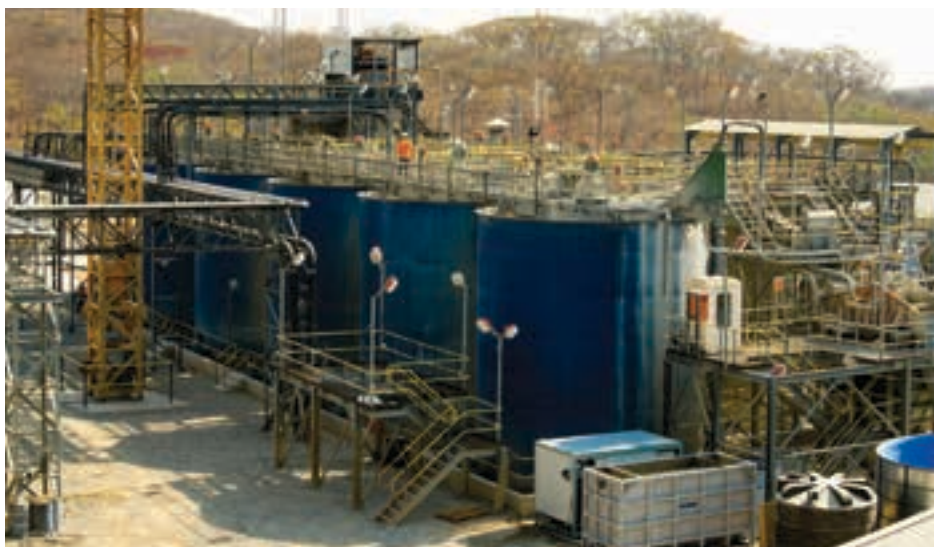
The CIL circuit at New Luika. The New Luika processing plant was commissioned in August 2012 with a new elution and electrowinning facility being added in Q2 2014 and a new crusher plant in September 2014.
