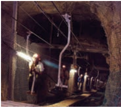
Becker Mining South Africa's chairlift systems are designed to transport up to 900 personnel per hour.
