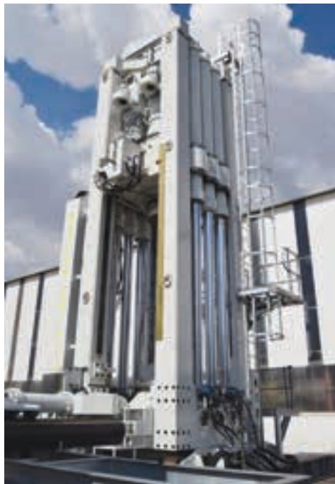
The RD8-1500, the largest raise bore rig in the world, was unveiled at Master Drilling's premises in Fochville on the West Rand earlier this year. The machine is now working at Palabora Mining Company's Palabora mine, where Master Drilling has a contract to deliver two 6,1 m diameter, 1,2 km deep ventilation shafts (photo: Arthur Tassell).
