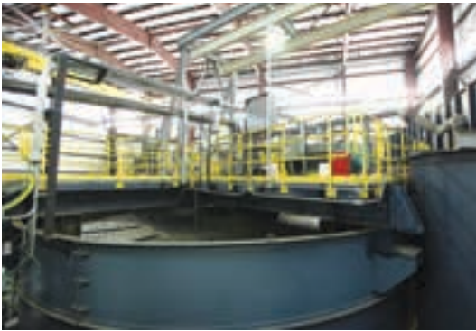
The new 600 Series SuperCell™ flotation machine is the world's largest operating flotation cell.
