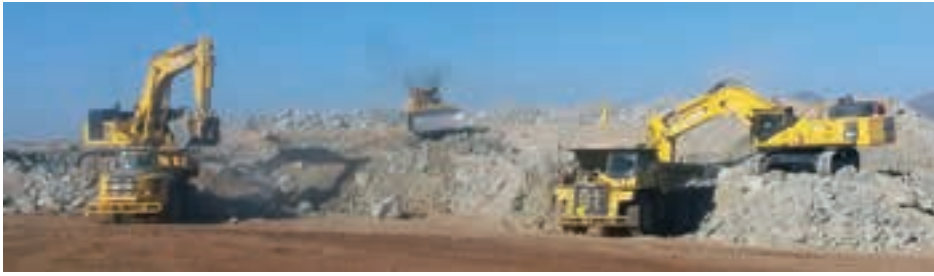
An example of load-haul operations. Concor Opencast Mining has both soft- and hard-rock operations.
