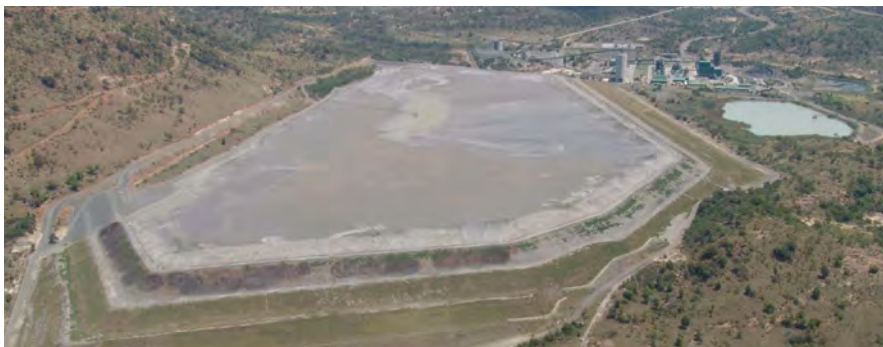
An aerial photograph taken of a tailings storage facility as part of an aerial inspection which forms part of an active monitoring program at the facility
