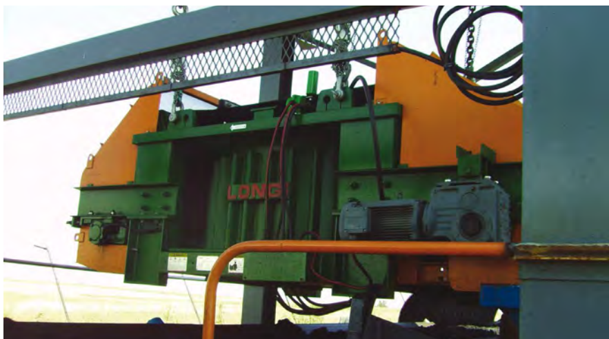
Longi-Multotec overbelt magnets are designed according to specific applications criteria.
