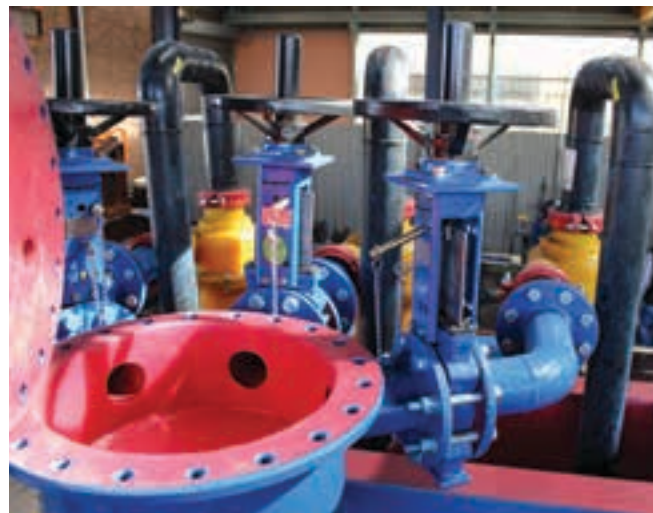
Below: Production of a three-way Cavex cluster incorporating Linatex premium rubber and Isogate knife gate valves.
