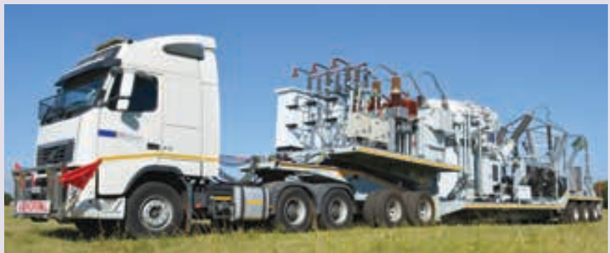
Overall dimensions and weight distribution are critical requirements in any mobile substation design. Zest Energy utilises a combination of a dolly trailer and the main substation trailer to conform to all legislative requirements governed by the South Africa Road Ordinance. Here shown is a 132 kV/88 kV/33 kV/22 kV, 40 MVA multi-ratio mobile substation set up for transport and ready for deployment to the operational site.
