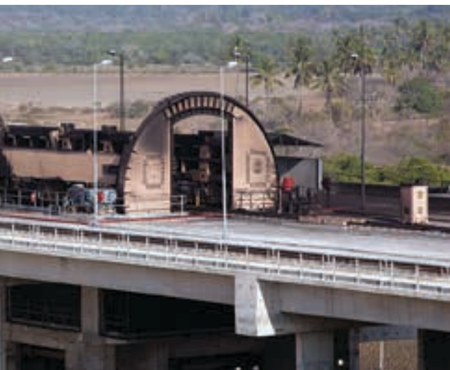
Above: ThyssenKrupp's most current success, a state-of-the-art ThyssenKrupp tandem rotary tippler at the Port of Nacala. These systems require deep bunkers underneath the rotary tippler to accumulate the material. Left: Rotary tipplers are designed so that the turning point coincides with the axis of rotation of the wagon couplings in the tippler. Right: Side tipplers are the simplest random tippler option.
