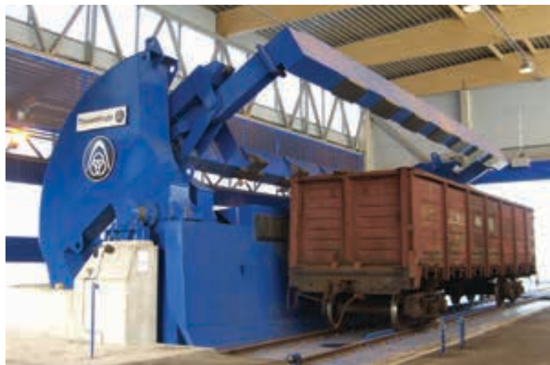
Above: ThyssenKrupp's most current success, a state-of-the-art ThyssenKrupp tandem rotary tippler at the Port of Nacala. These systems require deep bunkers underneath the rotary tippler to accumulate the material. Left: Rotary tipplers are designed so that the turning point coincides with the axis of rotation of the wagon couplings in the tippler. Right: Side tipplers are the simplest random tippler option.
