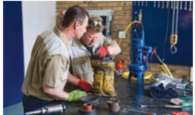
AESPUMP's dedicated workshop at its Secunda facility was commissioned to service pumps from Sundyne subsidiaries HMD and Ansimag. The new workshop is a 'clean-room' and supplements a separate, dedicated flame-proof pumps workshop.
