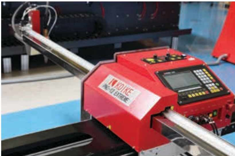
The PNC-12 Extreme from Koike, is an ideal entry-level CNC oxy-fuel or plasma cutting solution.
