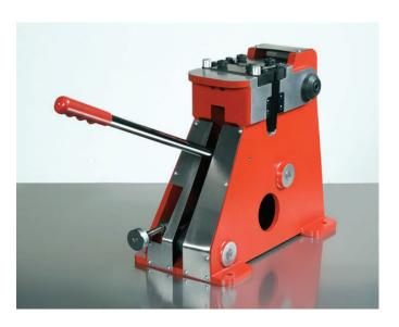
The smaller BM10 and BM30 manual welders, also for use on a workbench or with a trolley, are robust, durable machines with capacities ranging from 0.0039" to 0.071" (0.1mm to 1.8mm).
