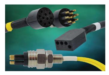
The new product series uses Amphenol's molding and adhesion expertise to offer an optional molded-to-cable feature. This feature ensures that the seal between the cable and connector remains intact under water. All polymer-to-metal bonding surfaces are carefully sandblasted, cleaned, primed and molded. The rugged metal shells and recessed pins assure reliable performance in the most demanding environments.
