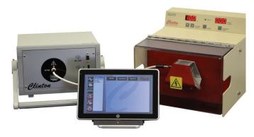
Clinton Instrument Company will display a new automatic spark test calibration system, the STCAL. This unit allows for quick and accurate voltage calibration of AC, both mains and high frequency, as well as DC units up to 30kV. It will calibrate spark testers from any manufacturer.
