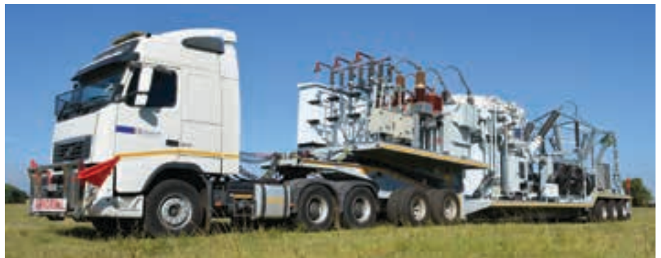
Overall dimensions and weight distribution are critical requirements in any mobile substation design. Zest Energy utilised a combination of a dolly trailer and the main substation trailer to conform to all legislative requirements stipulated by the South Africa Road Ordinance.
