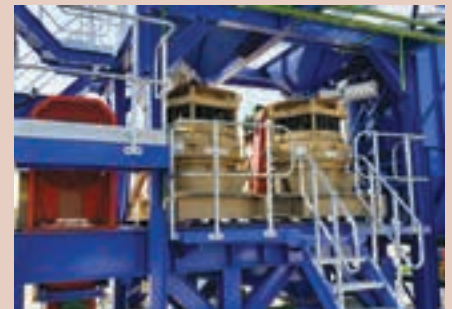
Gyrasphere cone crushers from Osborn installed at the Karowe diamond mine.
