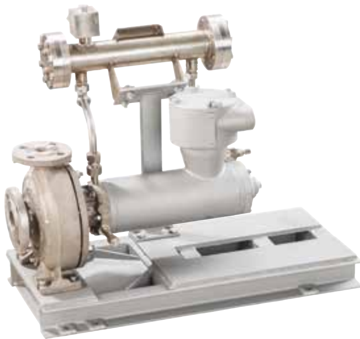
Ecochem HP variant has an integrated auxiliary hydraulic system that circulates the coolant and lubricant in the rotor space.
