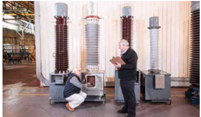
Nick de Beer (right), ACTOM HV Equipment's product manager, Instrument Transformers, with Jan Venter, supervisor (insulators) with one of the new 132 kV current transformers equipped with composite insulators and a new design secondary terminal block.
