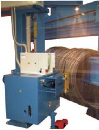
▲ The SS80 vertical butt welder from August Strecker
