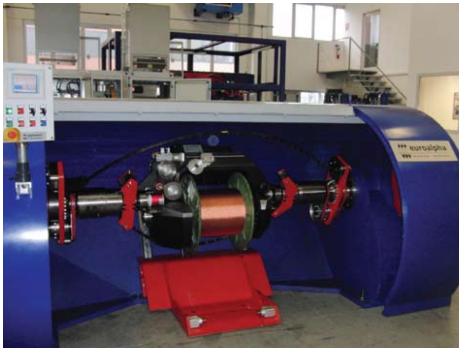
▲ Euroalpha's B630-F 'Four-Twist' bunching machine
