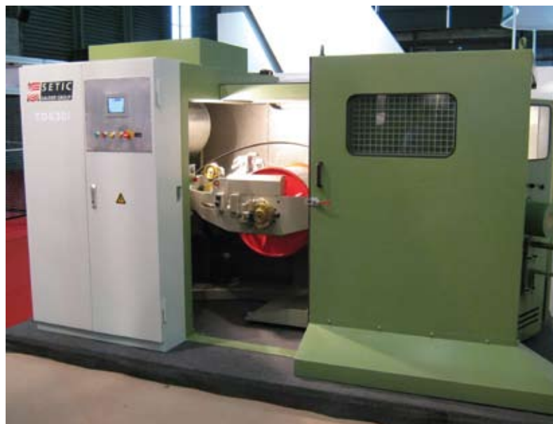
▲ SETIC double-twist bunching/stranding machine TD 630 i
