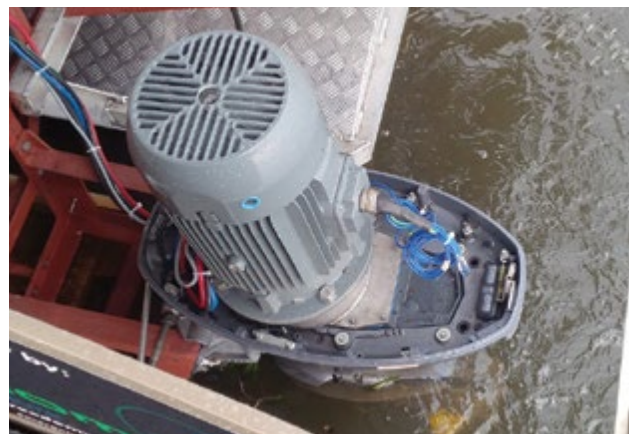
Figure 5: 30 kW WEG PM motor fitted to an outboard stem on the Chobe Game Lodge electric boat. (Cover has been removed for photo).
