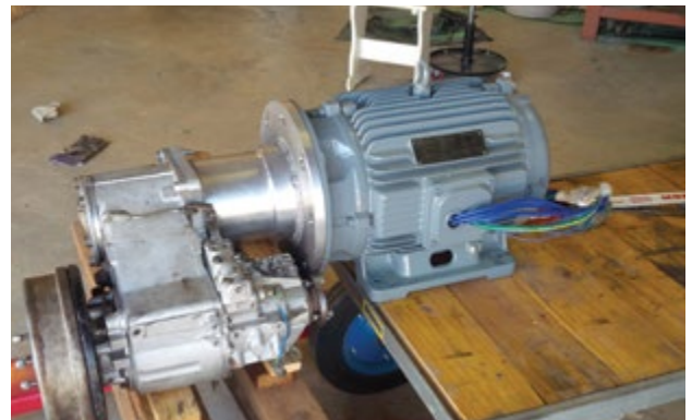
Figure 2: PM motor attached to the Land Rover Defender Transfer Case with a special adaptor housing ready to be installed into an EV Conversion.
