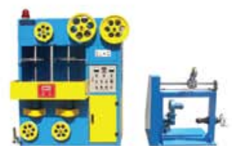
Ø630/Ø800 单层、双层、三层包纸机(绕包机) Ø630/Ø800 Single layer or double layers or three layers wrapping machine
