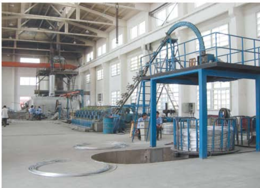
Aluminum Rod Continuous Casting & Rolling Line Type ZZR1500+255/15
