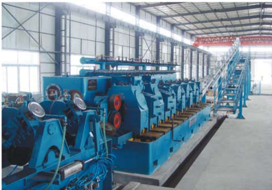
Copper Rod Continuous Casting & Rolling Line Type ZZR1800+255/12
