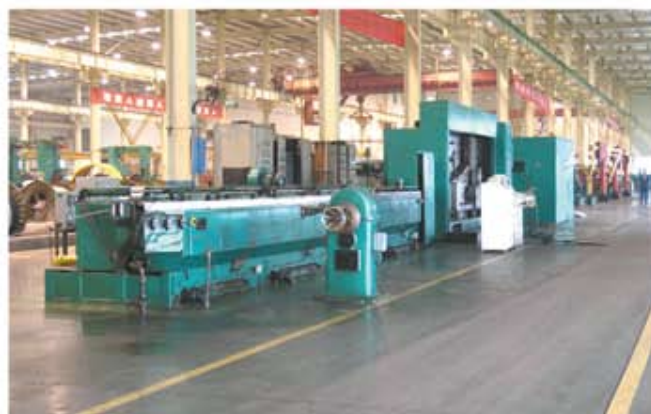
Copper Rod Breakdown Machine Type LHD450/13T with Continuous Annealer
