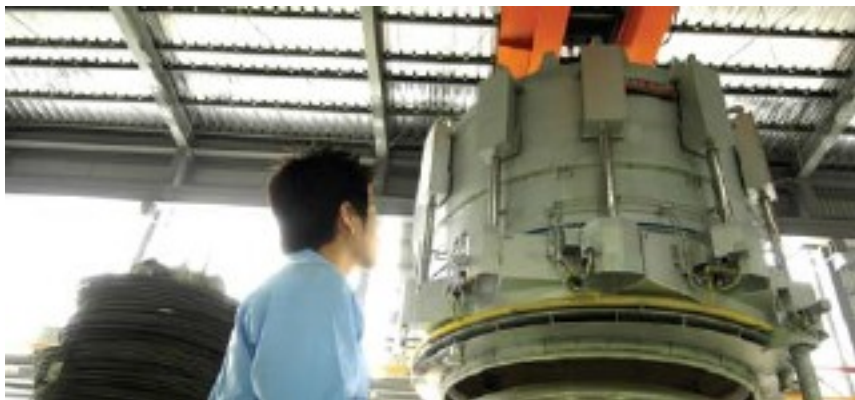
○ Rad-Con's 100% hydrogen super-high convection bell-type annealing furnace
