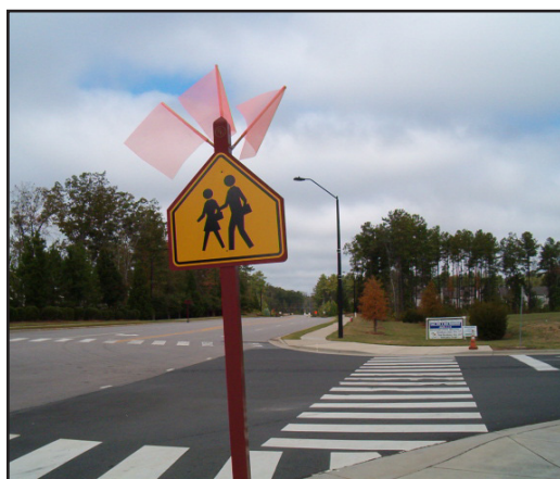
High-Visibility Crosswalk in front of Cedar Fork Elementary.
