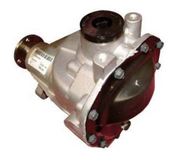
In vehicles, the differential allows the outer drive wheel to rotate faster than the inner drive wheel during a turn. This is necessary when the vehicle turns, making the wheel that is traveling around the outside of the turning curve roll farther and faster than the other. The average of the rotational speed of the two driving wheels equals the input rotational speed of the drive shaft. An increase in the speed of one wheel is balanced by a decrease in the speed of the other.
