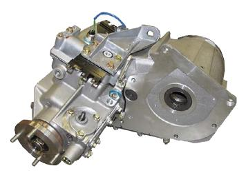
Transfer boxes that are designed to allow for normal road use synchronize the difference between the rotation of the front and rear wheels, in much the same way the differential acts on a given axle/diff. This is necessary because the front and rear tyres never turn at the same speed. Different rates of tyre rotation are generally due to
