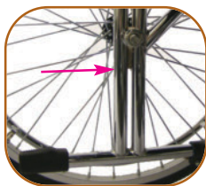
Double Bar Vertical Reinforcements
