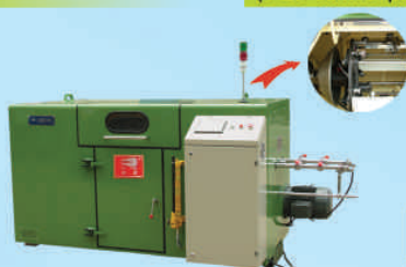
HD- \phi 300B- \phi 630B Hi-speed automatic single strander, twister series (PLC control panel)
