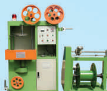
\phi 630- \phi 800 single layer super-hi-speed paper wrapping machine
