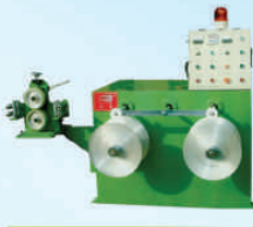
HD- \phi 400 cross coiling machine
