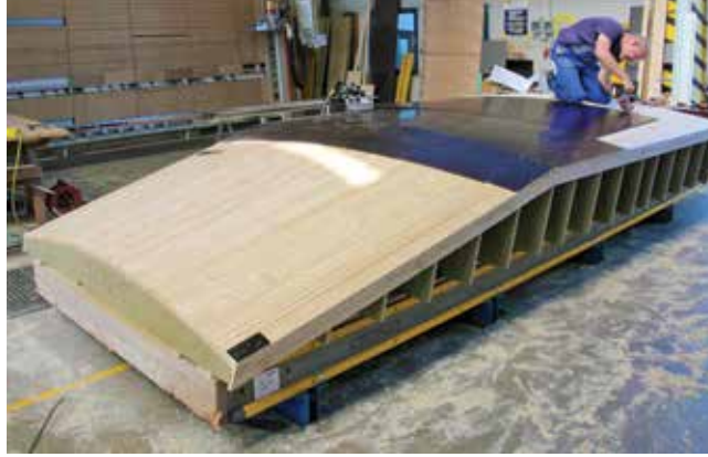
ABOVE: All of the assembly work for these highly sophisticated formwork panels is completed at the Doka Pre-assembly Service. BELOW: Fine adjustments are accomplished by using top-mounted forming boxes. Photos: Doka
