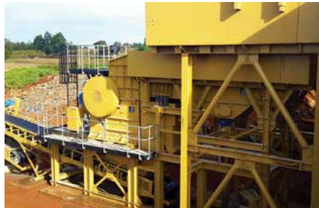
The modular design of the Trio jaw crusher provides extra value by reducing transportation and installation costs.
