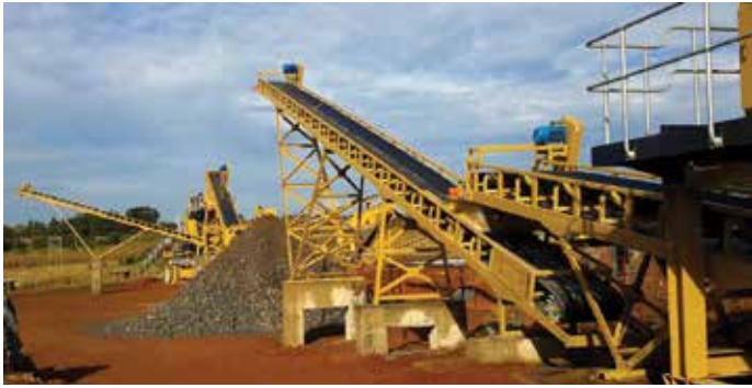
A 250 tph modular Trio aggregate plant installation in East Africa.
