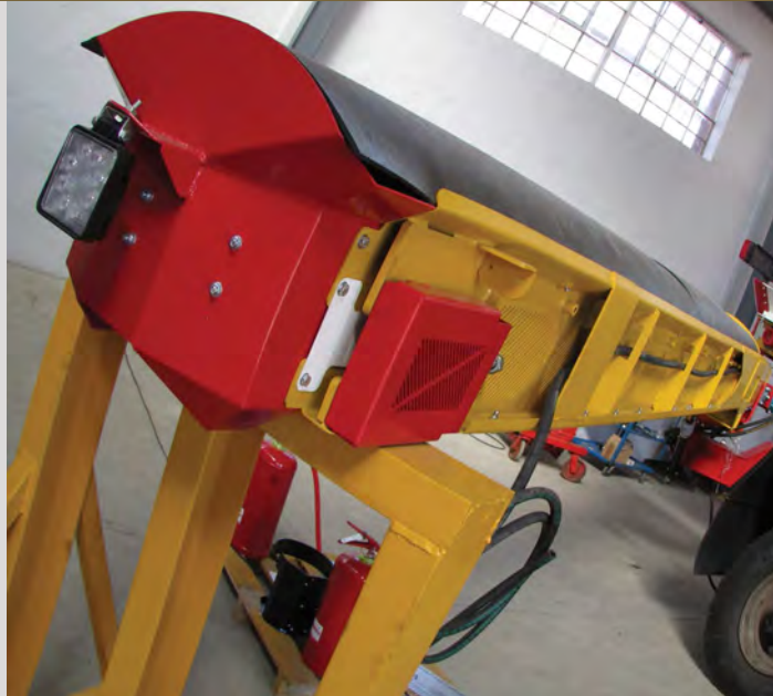
All trucks are fitted with an eight metre boom conveyor (170 degrees). Karel Steyn, technical manager at Cobra Petro Projects.
