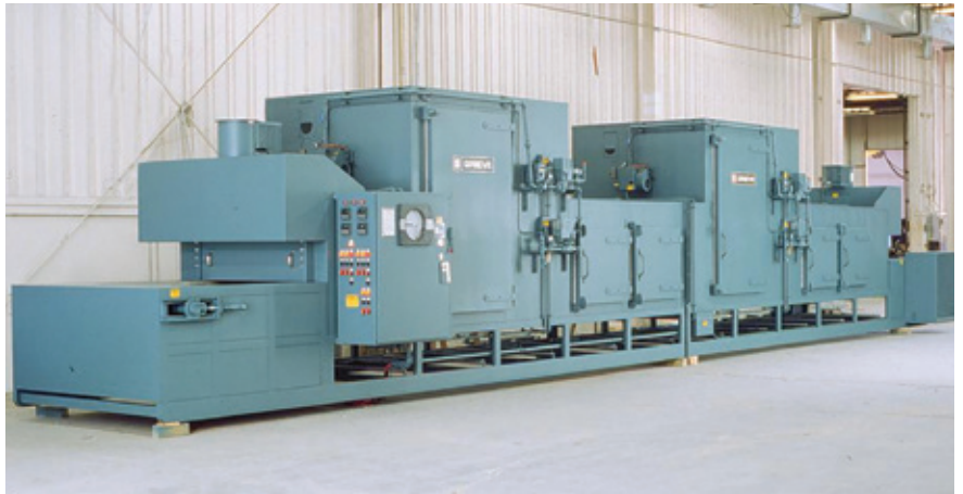
▲ The unit has a maximum operating temperature of 850°F
