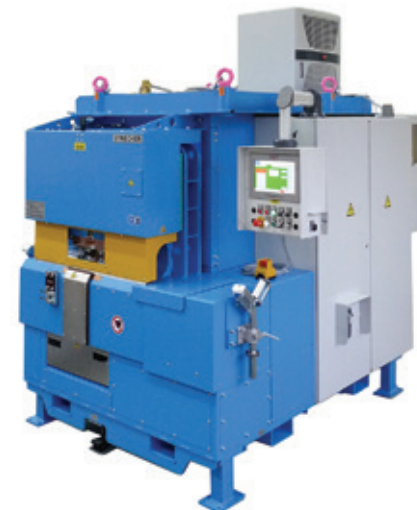
▲ The MK1200 for welding copper or aluminium stranded conductors up to a maximum of 2,500mm 2
