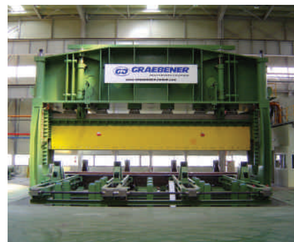
Ⓢ A JCO pipe forming press from Graebener
