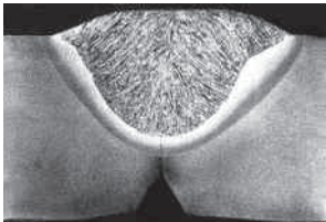
Continuous submerged-arc inside welding
