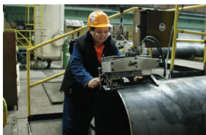
The process of stamping on spiral welded pipe
