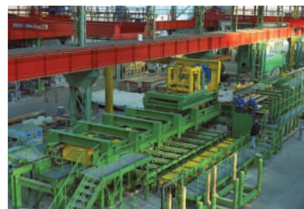
Ⓜ A 3,000kN tube-drawing bench
