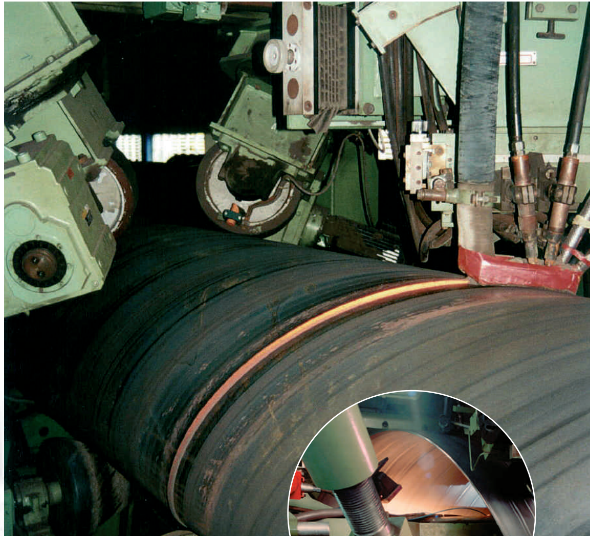
Complete submerged-arc inside and outside welding seam
