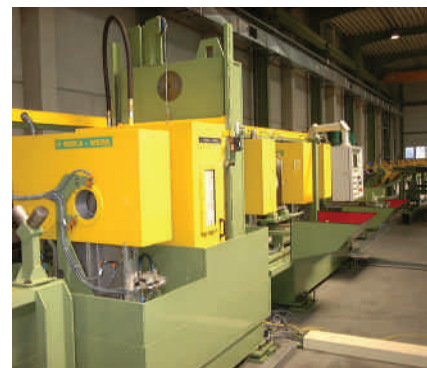
Reika's turnkey NDT system for seamless steel tubes
