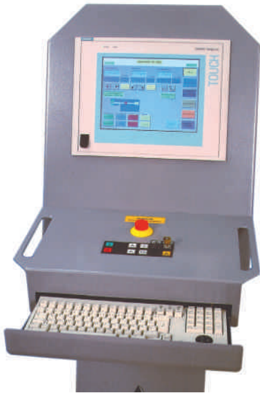
① All integrated manufacturing cell components are operated via a Simatic panel PC with touch screen and menu-driven user-guidance
