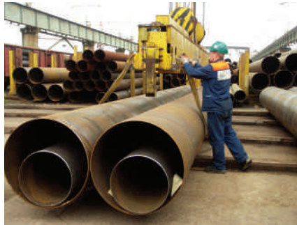
US Steel Košice manufactures spiral welded pipes from Ø 406mm to 1,420mm
