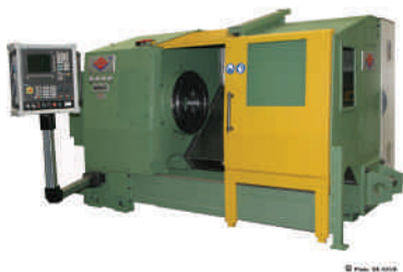
Model MPM-C7 coupling finishing machine (60.3-177.8mm)
