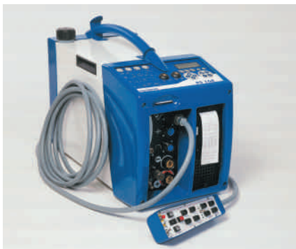
🔧 The portable orbital power source used by Idroinox
