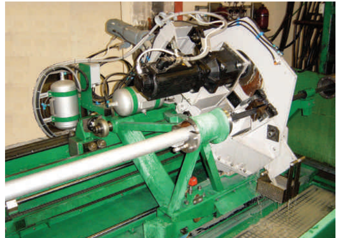
Figure 1: A detail of a sawing unit KS 76x3.4 with flying saw cutoff – ALDAS
