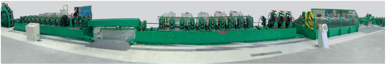
Figure 7: A fish eye view of an Attl mill for tubes to 104x4mm
