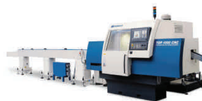
Ⓢ Sinico's Top 1000 CNC automatic cutting and bar end-working machine
