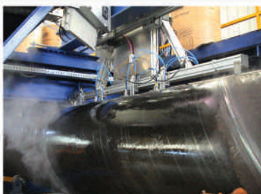
ULTRASONIC TESTER UT MX SAW SPIRAL & ERW Up to 32 Channels – Real Time Strip-Chart Full trace ability
