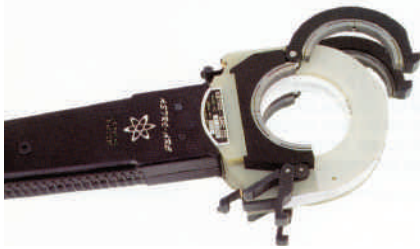
🔧 Closed welding 'K-Series' head, adapted to titanium applications in the aerospace industry
