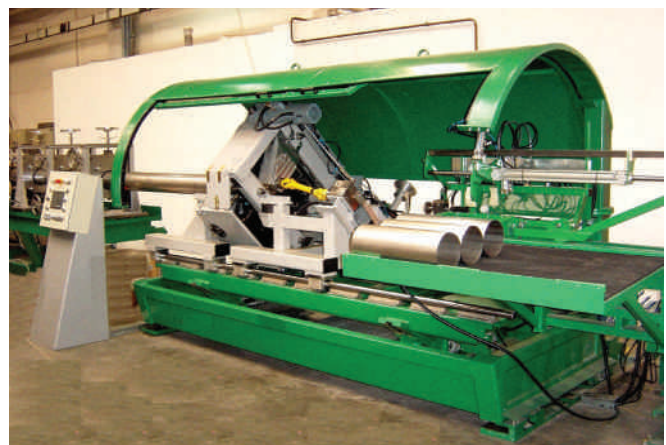
Figure 6: Flying saw cutoff ALDAS 200x6-40-Kvatro
