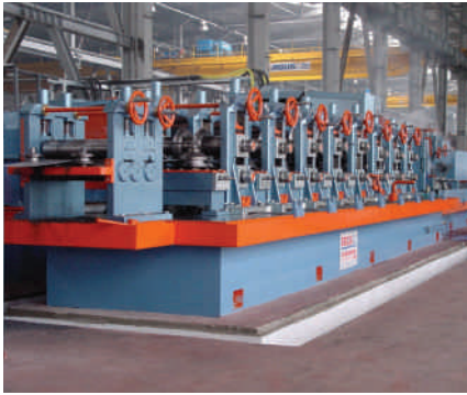
A mill for the production of welded tube
