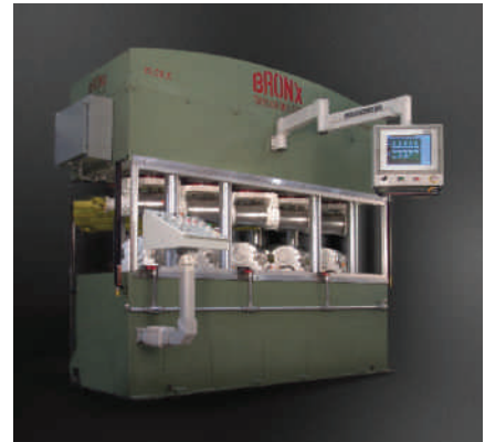
Bronx/Taylor-Wilson's tube straightening machine is available in 6 and 10 roll configurations
