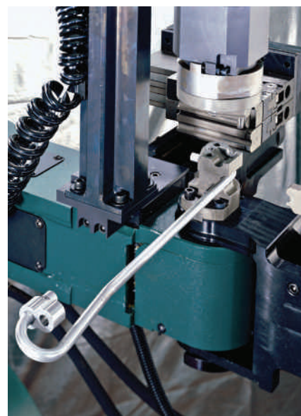
The working area of the BLM Dynamo MR200E five-axis CNC tube bending machine, recently installed in Team Precision Pipework's South Wales factory
