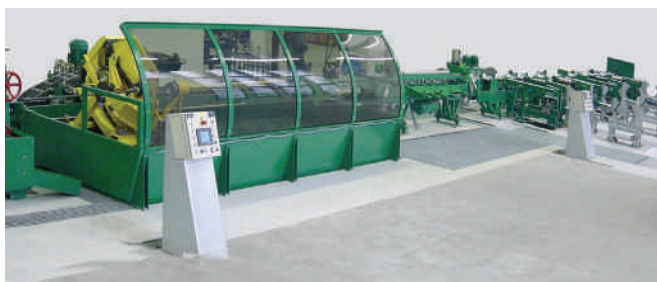
Figure 3: Flying saw cutoff ALDA S 76x3.4-100, with AUT 7000 bundling machine shown in the background
