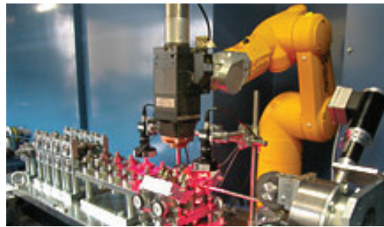
Metal forming bench and robotic laser welding arm
