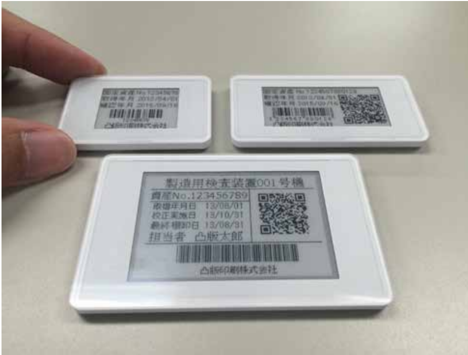
Figure 2: Toppan’s batteryless EPD with built-in RFID tag (Source: Toppan Printing)
