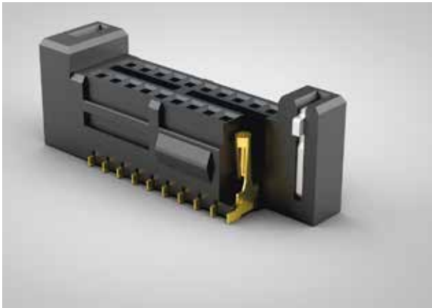
Rugged design features can make micro pitch interconnects rugged by incorporating BeCu contacts, weld tabs, latches, and locks
