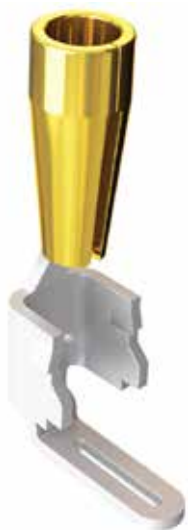
Multi-finger, heat treated BeCu contact for high cycle, high reliability applications
