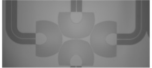
Figure 3: Focusing grating couplers can send the light in waveguides outward from the surface, enabling them to efficiently illuminate the cells in the microfluidic channel located above
