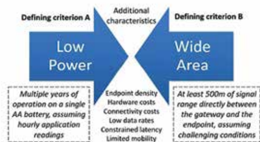
Figure 1: Definition of a LPWA network – Machina Research.
