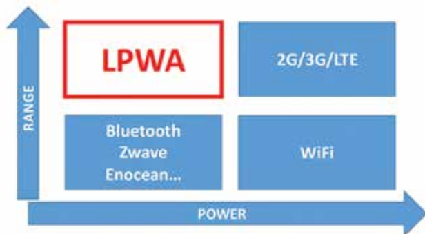
Figure 3: LPWA networks address the need for ubiquitous long range, low-power communication.
