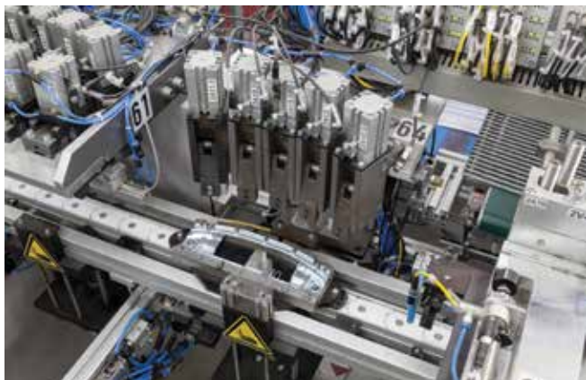
Figure 3: Fully automatic assembly of a vacuum cleaner nozzle at several stations.
