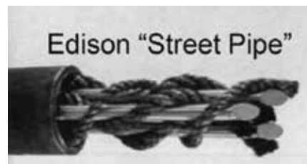
Figure 1: First power cable – developed by Thomas Edison in the early 1880s.
