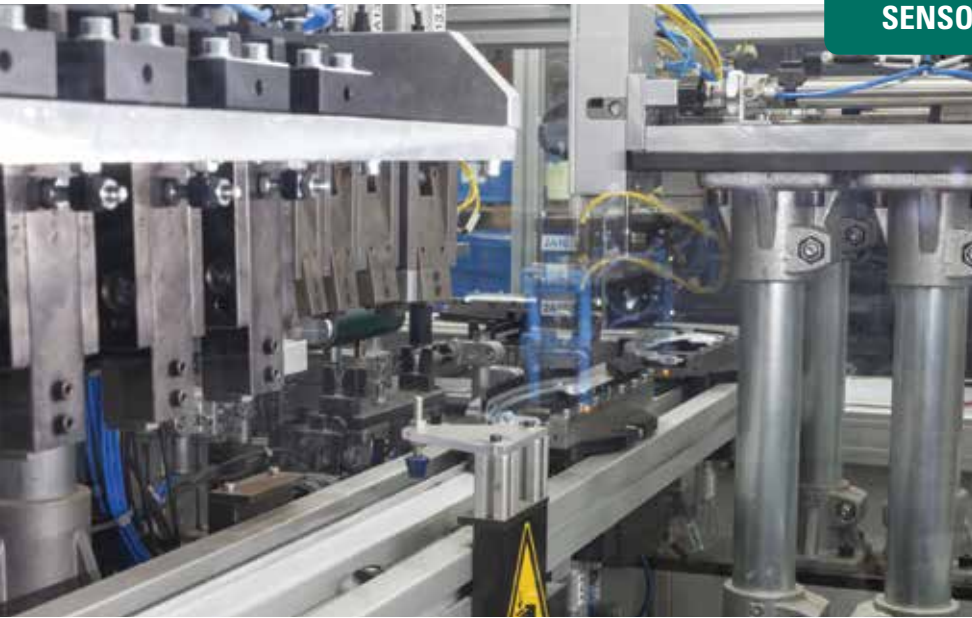
Figure 2: Assembly machine for the production of vacuum cleaner nozzles.
