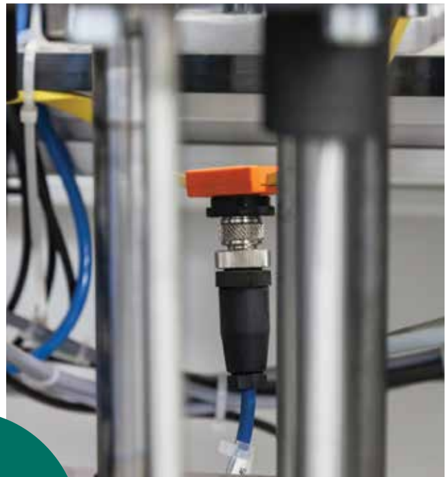
Figure 5: Sensors can be connected to any spot of the AS-i cable via a flat cable insulation displacement connector.
