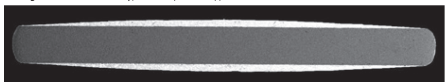
▼ Figure 3: Cross-section of a typical hot-dip tinned copper ribbon
