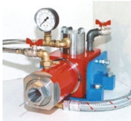
▲ Wire cleaning by PWC system
