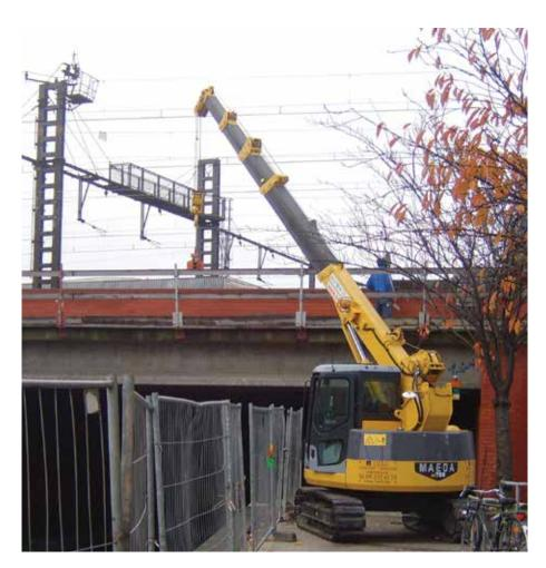
tional tyres or tracks. A major feature of the Maeda Mini Crawler Cranes is the boom construction. The pentagonal shape of the boom increases the strength and prevents unnecessary flexing in extreme conditions. The smaller units are fitted with a four stage boom whilst the larger units have the additional fifth stage.
