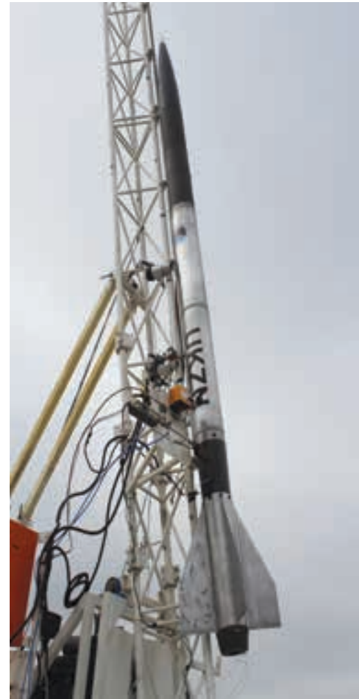
The Phoenix-1A hybrid sounding rocket immediately prior to launch at the Overberg Test Range.
