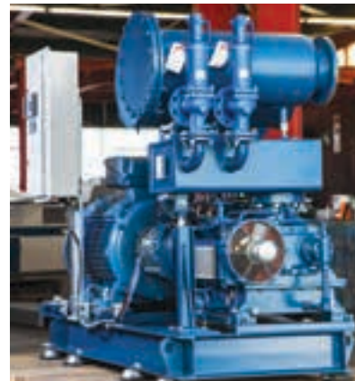
An Aerzen Delta Screw, oil-free screw compressor.
