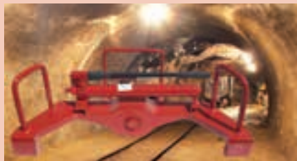
Becker Mining South Africa's hydraulic rail benders, which bend and form rails on railway lines in heavy industrial and underground transport systems on the mines, easily handle rail of up to 40 kg/m.
