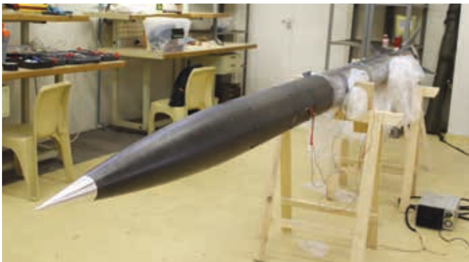
Under development, UKZN's aerospace Group's Phoenix-1A, a hybrid rocket with a theoretical apogee of 10 km, capable of delivering a payload of 1.0 kg.
