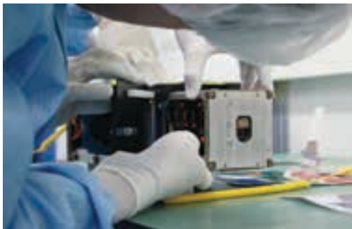
TshepisoSAT, South Africa's first nanosatellite, is a tiny 1,2 kg cube satellite measuring 10×10×10 cm.
