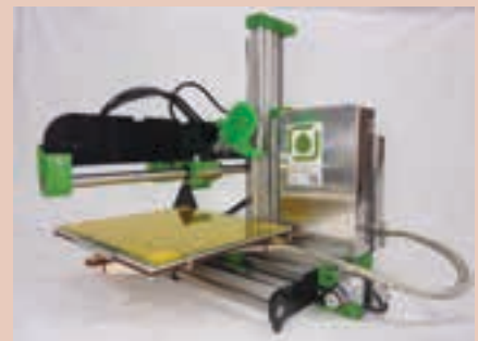
The fully assembled RepRapPro Ormerod 2 3D printer, now available in kit form in South Africa from RS Components (RS), offers build volume and speed of 200×200×200 mm and 1 800 mm/min, respectively; accuracy of 100 µm and layer resolution of 10 µm.
