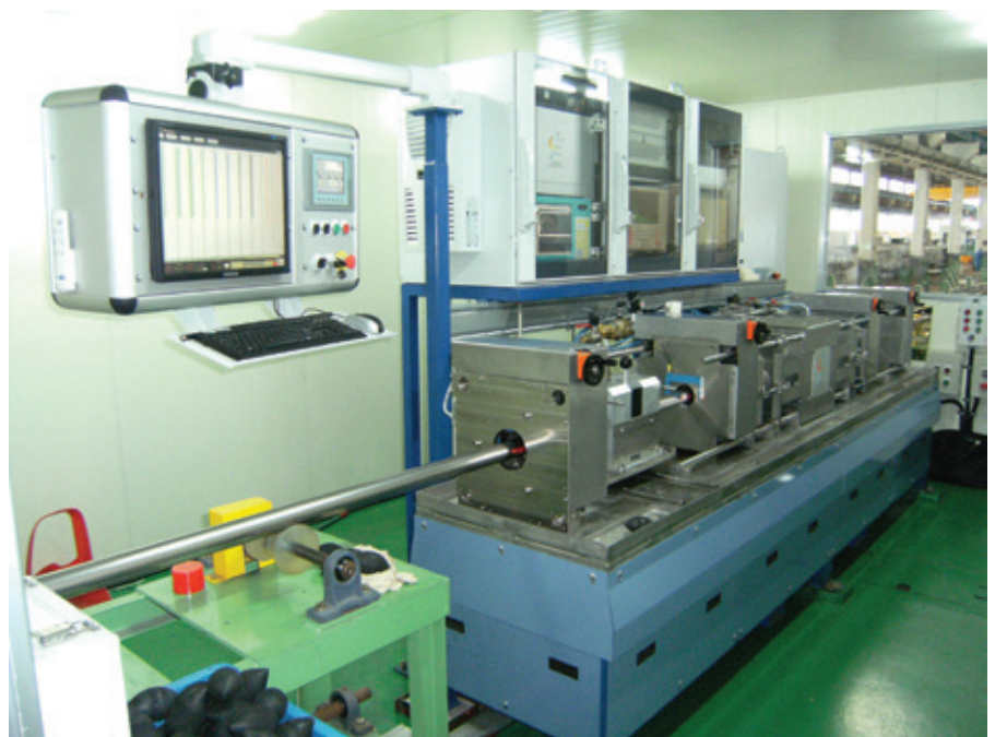
RotoUTscan ultrasonic rotating head
