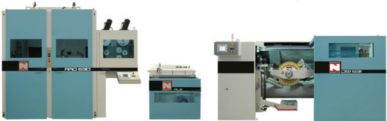
○ DSI pairing line consisting of an ARD 630 double twist backtwist pay-off, an ALB longitudinal tape pay-off and a type DSI 631 double twist stranding machine
