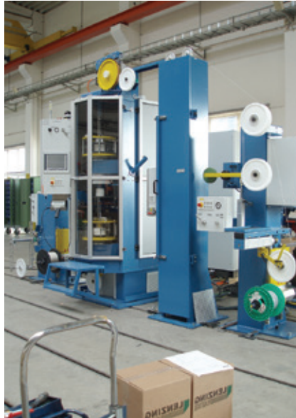
○ A vertical taping and sintering line for aircraft cables
