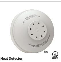
Heat Detector connects easily to most commercial fire alarm systems. For use in areas where property protection is required such as boiler rooms, kitchens, medicine or linen storage areas. Rate-of-rise models respond to a temperature increase of 15° F/minute, sensing flash fires even before the 135° or 194° fixed temperature is reached.
