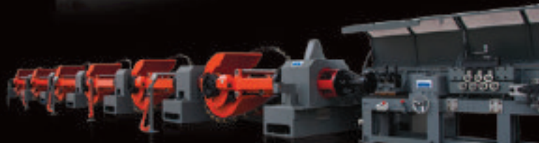
PC-Wire and PC-Strand production lines
