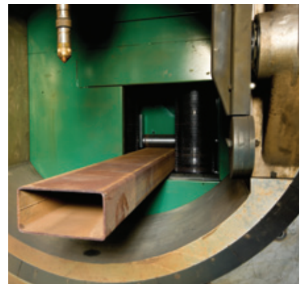
Drilling rectangular tubing
