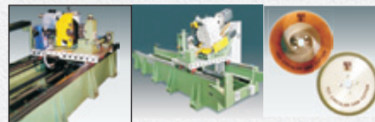
Burr free cold saw fly cut off
