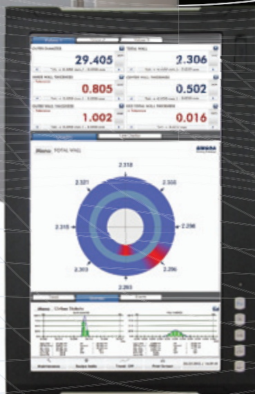
ECOCONTROL 6000 displays production data of the X-RAY 6000 PRO
