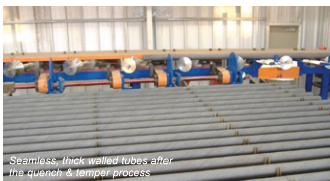
Layout of a typical induction equipment for heat treating of tubes (Quench & Temper)
