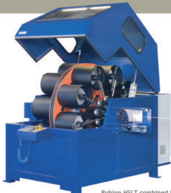
Roblon HSLT combined high- speed, low-tension server
