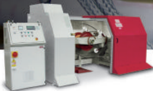
BM 800 Double-twist bunching machine
