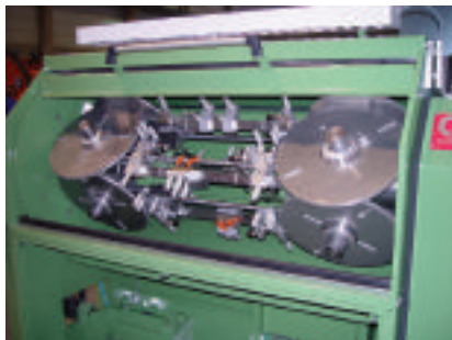
○ The newly-designed 8-pad taping head for rectangular copper wires
