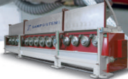
MT 500 Aluminum wire rod break-down machine
