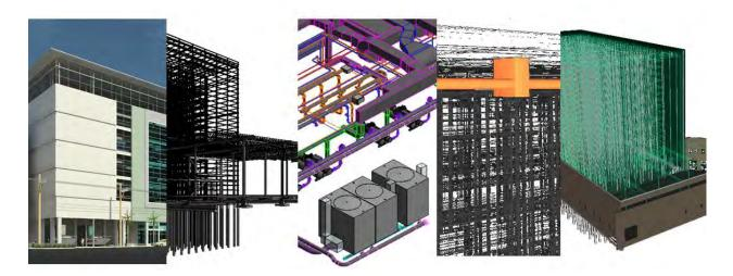
BUILDING INFORMATION MODELING OR BIM IS THE PROCESS OF DEVELOPING A VIRTUAL BUILDING MODEL THAT ALLOWS THE PROJECT TEAM TO SEE, INTERACT, ANALYZE AND COLLABORATE IN AN INTELLIGENT 3-DIMENSIONAL ENVIRONMENT. J. RAYMOND CONSTRUCTION ADOPTED THE USE OF BIM IN 2011. BENEFITS FROM BIM IMPLEMENTATION WERE IMMEDIATELY RECOGNIZED WITH A REDUCTION IN THE NUMBER OF RFIS, COSTS AND TIME DELAYS.
