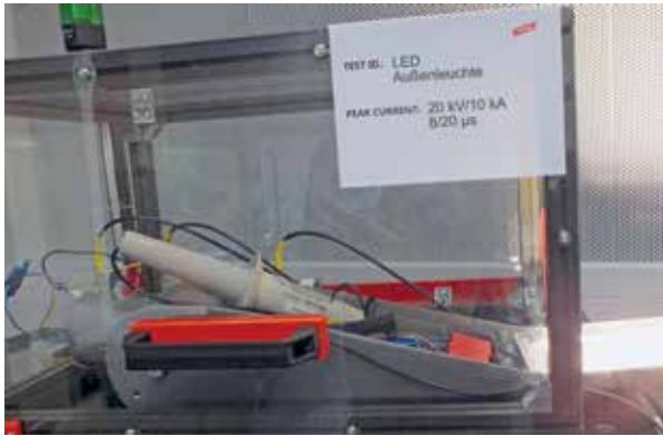
Figure 7: Test set-up for a complete LED street lighting system in the laboratory.
